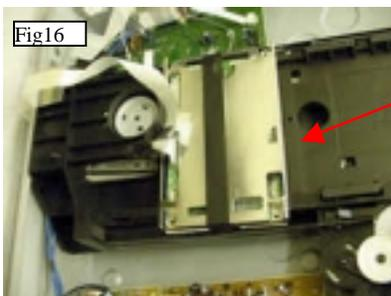
If the shorting PCB seen in Fig 3 is not in place, you will need to keep the DSP still connected to CN501 connector until pick-up shorting is done as seen on figure 10. Keep DSP attached to the frame with an electrical tape.
