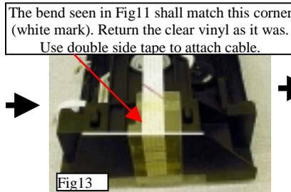
Re-assemble the unit back and attach the cable as illustrated next Fig14. It is important to keep the pickup shorted until last.
